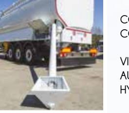
COCLEA AUTO-CARICO mt 4 CON MOTORE IDRAULICO
